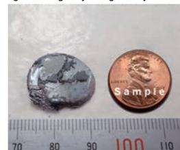
Large SnS single crystals grown by flux method
