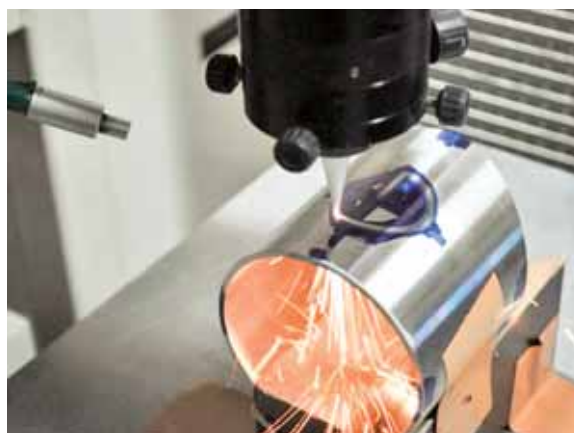
YAG laser cutting process
