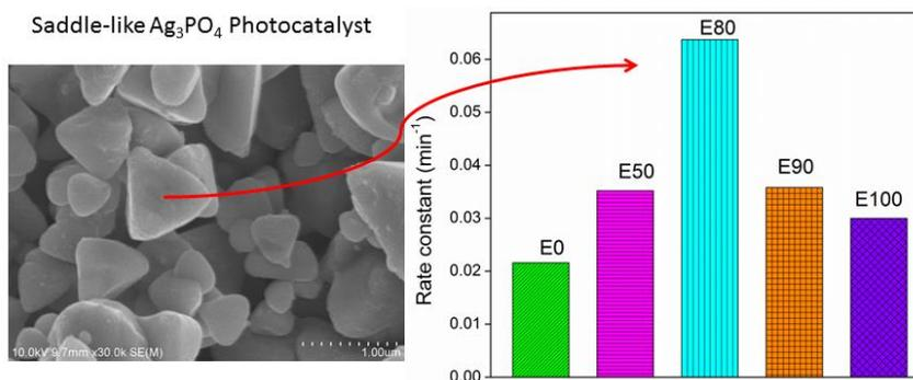
Fig1. Photocatalytic activities of the  $\text{Ag}_3\text{PO}_4$  synthesized using  $\text{H}_3\text{PO}_4$  ethanol solution and  $\text{AgNO}_3$  ethanol-aqueous solution with the ethanol contents (v/v) of 0% (E0), 50% (E50), 80% (E80), 90% (E90) and 100% (E100) [3].
