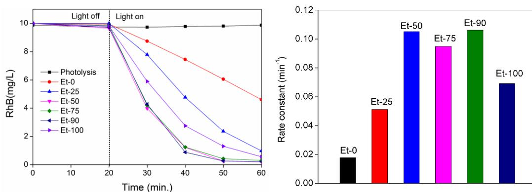
Fig. 2 The photocatalytic activities of  $\text{Ag}_3\text{PO}_4$  synthesized using  $\text{Na}_2\text{HPO}_4$  aqueous solution and  $\text{AgNO}_3$  ethanol-aqueous solution with the ethanol contents of 0% (Et-0), 25% (Et-25), 50% (Et-50), 75% (Et-75), 90% (Et-90) and 100% (Et-100).
