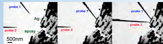
Conductivity measurement process utilizing the double-probe piezodriving holder.
